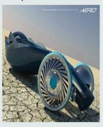
The green vehicle has its body made of compressed polymers that considerably reduce the weight of the car and which can be easily recycled. Each of the two front wheels of AERO has its own electric motor that is linked to the car's steering wheel via a wireless system. The onboard batteries can be recharged using the power of wind and sun, plus one can plug the car into a 120V source.
